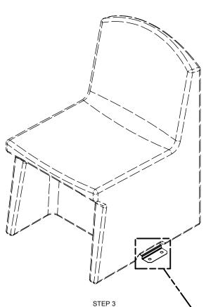
Place the chair with the bolt down plates at a desired location and mark the hole locations. Move the chair aside and place the anchors in the marked locations. Place the chair back into anchor locations and secure the mounting plate to the floor.
