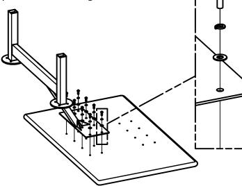
**Step 1 - ADA Bolt Down Version Only** After securing Leg Frames, secure Oasis ADA Leg to ADA Table Top using (4) 5/16-18 x 1-1/4 FH Screws.
