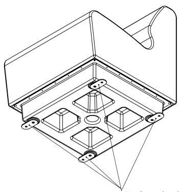
Mark anchor locations on floor and secure the chair to the floor with the bolt down tabs using mounting hardware.
