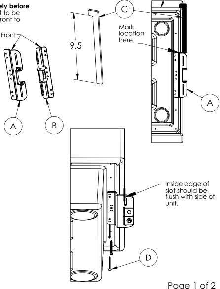
Rev. B - 4/9/14 091-854 Typically, the bracket with the tabs (B) should be attached to the unit that will be on the right.
