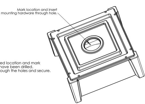
Step 2: Place Base at a desired location and mark them through the holes that have been drilled. Insert mounting hardware through the holes and secure.
