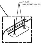
**NOTE: EACH MOUNTING PLATE COMES WITH 2 MOUNTING SCREWS**
