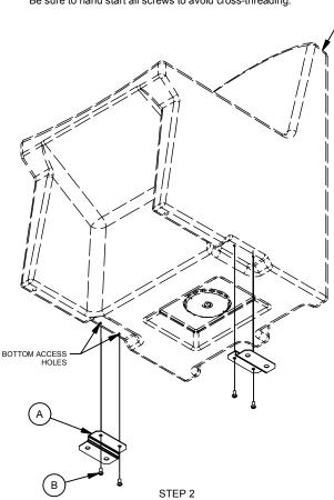
Attached the Mounting Plate (A) with the Seat Mounting Holes to Bottom Access Hole of the Chair using (2) 1/4-20 Button Head Screws (B) as shown. Repeat for other Bottom Access Holes.
