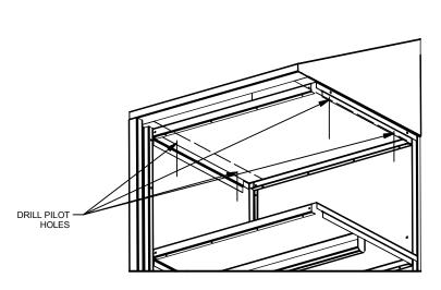
STEP 1: Line up the sloped top with the front and sides of the wardrobe
