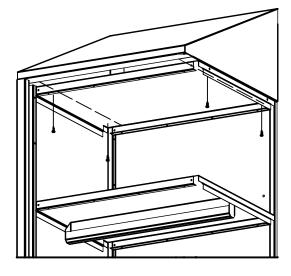
Drill (4) pilot holes in the top of the wardrobe that will line up with the sides flanges on the sloped top.
