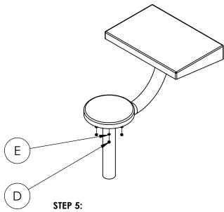
Secure Seat with (4) 5/16 Lock Washers (E) and (4) 5/16-18 Nuts (D). If you are using Slammer Stone Seats, secure the seat with (4) 5/16-18 Flat Head Screws (k).
