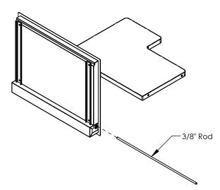
**Step 3:** Reinsert the 3/8" Rod Through Housing and Seat.
