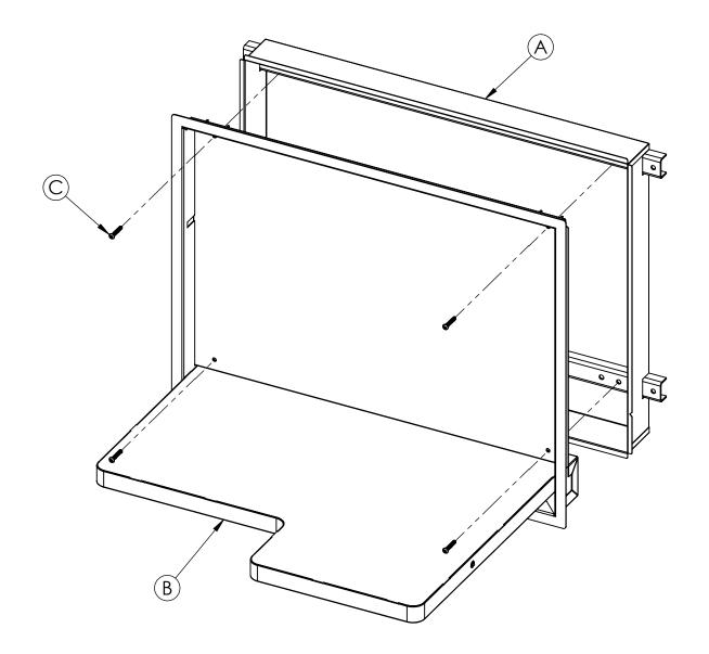
\*WALL MOUNT ASSEMBLY INFORMATION Wall Mount Assembly must be securely anchored to supporting wall to function properly.
