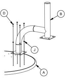
and secure the Leg to the Top using (4) 3/8 Lock Washers (J) and (4) 5/16-18 Screws (D). Repeat for each leg.
