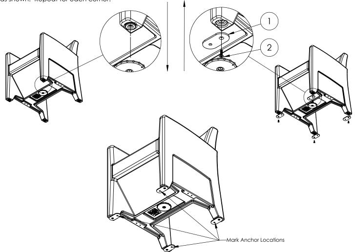
STEP 3: Mark Anchor Locations to the floor and secure the chair to the floor with the bolt down tabs using mounting hardware.
