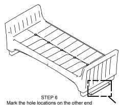
Mark the hole locations on the other end of the Sleigh bed (A) with the Mounting Plate (B). Move the bed aside and install the anchors in marked floor. Move the bed back into place, engaging the Secure Bracket at one end and securing the Mounting Plate to the anchors on the other end.
