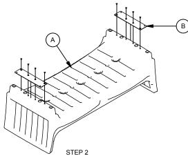
Turn the Sleigh Bed (A) upside down on a protective surface. Attach (2) Mounting Plates (B) on each end of Sleigh Bed with the countersink facing out using (8) 5/16 Flat Head screws
