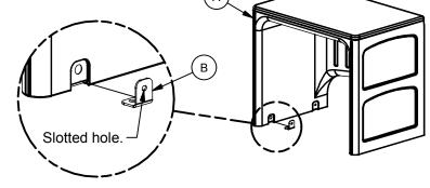
3. Place masking tape on the floor along the edge of each bracket, as shown, and mark the edge and ends of the brackets.
